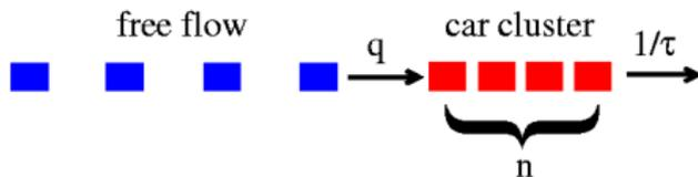
$q$  [veh/h] = traffic flow or traffic volume (from net time gap for a freely moving car)
