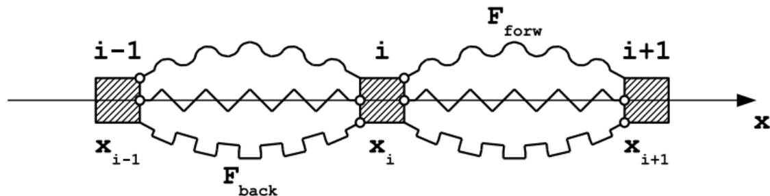
**Abb.:** A chain model of particles coupled by springs. The forward- and backward-directed forces are represented as different springs marked by  $F_{\text{forw}}$  and  $F_{\text{back}}$ , respectively. Each of such springs connects two particles, but acts only on one of them – that particle for which the connection is marked by a circle. The zig-zag spring in the middle shows the usual symmetric interaction.
